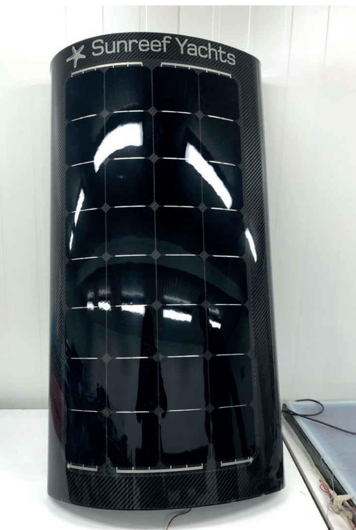
Carbon mast with in-built solar panels
