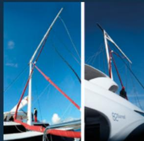
Sunreef Yachts launches the world's first catamaran-superyacht with a folding mast. Engineered and produced by Sunreef Yachts, the carbon fiber mast folds forward in its middle section at a 90 degree angle.
