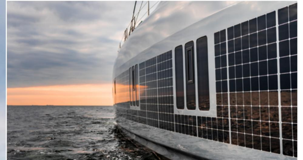
Thanks to their advanced integration technique, Sunreef Yachts Eco solar panels have a very high resistance to shock and abrasion. The catamaran was also fitted with a powerful custom-engineered battery bank.
