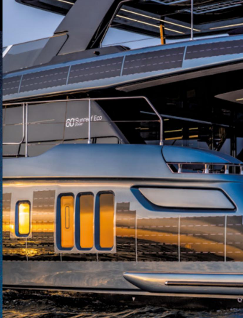
The luxury 60-footer is equipped with the shipyard's revolutionary solar power system with photovoltaic cells built into the yacht's hulls, bimini roof and superstructure. The green energy generated powers both the propulsion and appliances on board.
