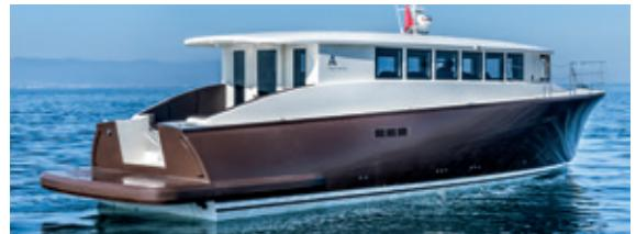
► **The Turkish yard has launched a taxi limousine of 16.85meters long, 475 centimeters wide, which can seat up to 36 people. With two Volvo Penta engines of 725 hp each it reaches a top speed of 31 knots. The cruising speed range is of 330 nautical miles.**
