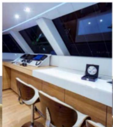
Diana has everything she needs to conquer the world's oceans. Her rigging includes a carbon mast and an in-boom furling system. The main navigation station is equipped with touchscreens enabling automatic sail adjustments coupled with load sensors to prevent wind, hardware and rig overload (for those who might be worried about accidental or uncontrolled gibe). These solutions provide a redundant, easy and safe control of the sails and rig.
