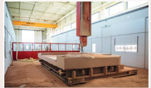
Europe's largest CNC milling machine in action. It is used to shape giant molds.
