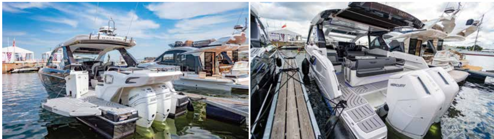
Galeon's 325 GTO (left) with twin 350hp Mercury outboards; the 375 GTO (right) with two 600hp Mercury V12 Verado engines
