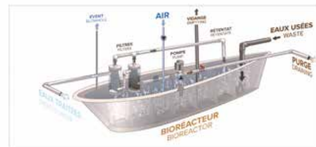
Bali is implementing a submerged membrane bioreactor on its models to sterilise all waste water on board and discharge totally depolluted water
