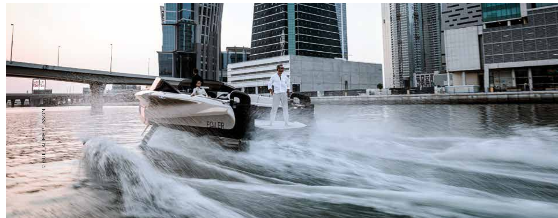
Built by Enata in the UAE, the 40-knot Foiler has been billed as 'The Flying Yacht' due to four foils that lift it up to 1.5m above the water, providing great stability
