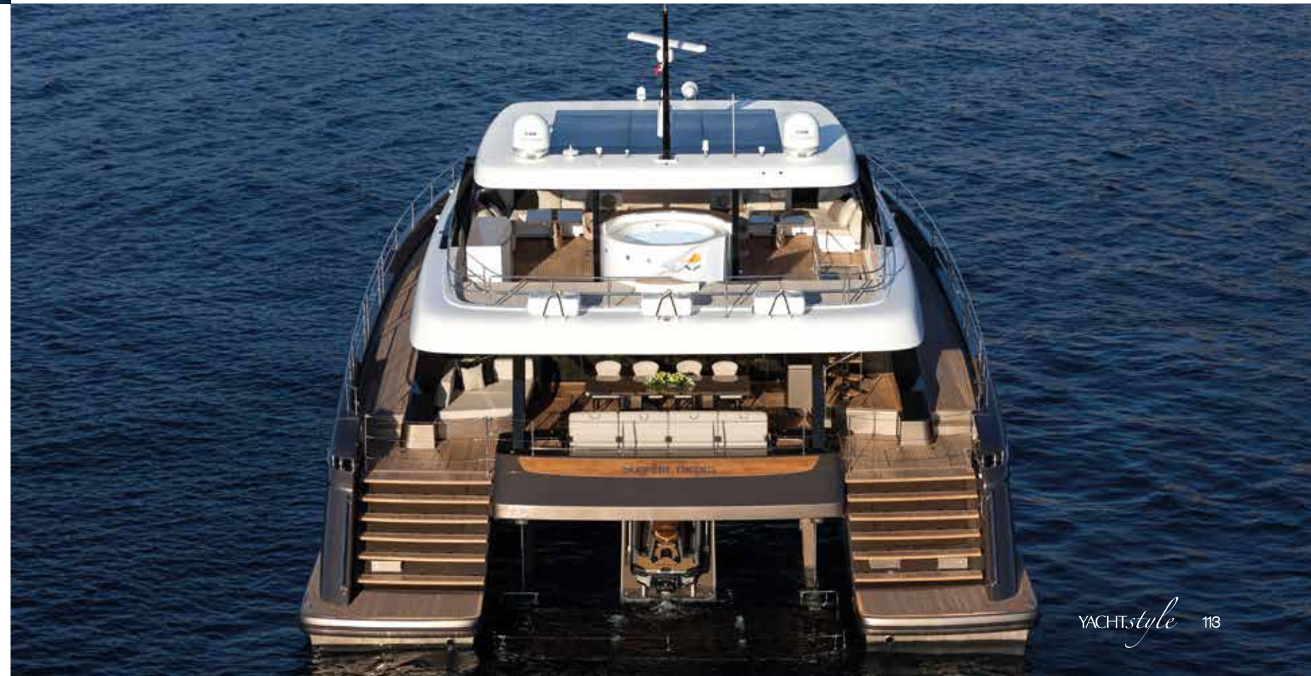
The innovative jetski 'garage' sits under the aft cockpit sofa, which can be raised upwards and aft to allow access
