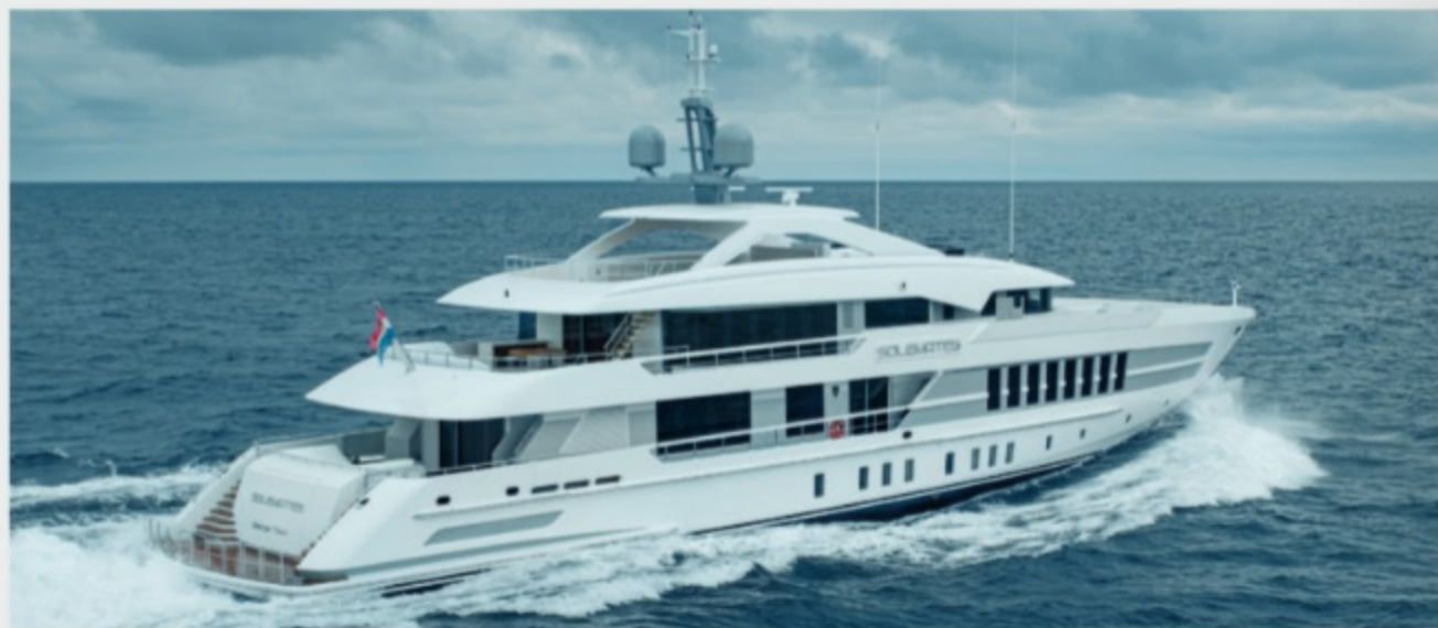
Latest Heesen 55m Steel Class has six staterooms on three decks, and uses the ultra-efficient fast-displacement hull form devised by Dutch hydrodynamicists van Oossanen
