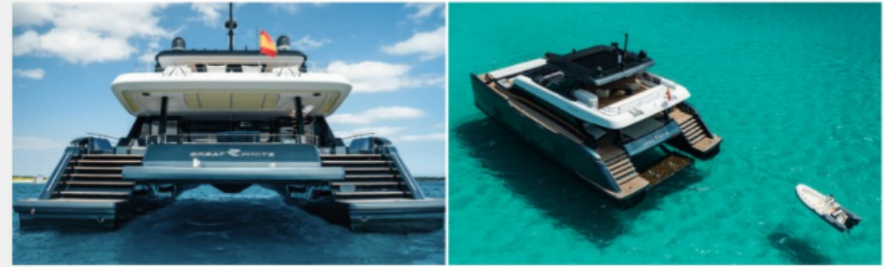
The hydraulic swim platform carries and deploys Nadal's tender, while the jetski is carried under the aft cockpit
