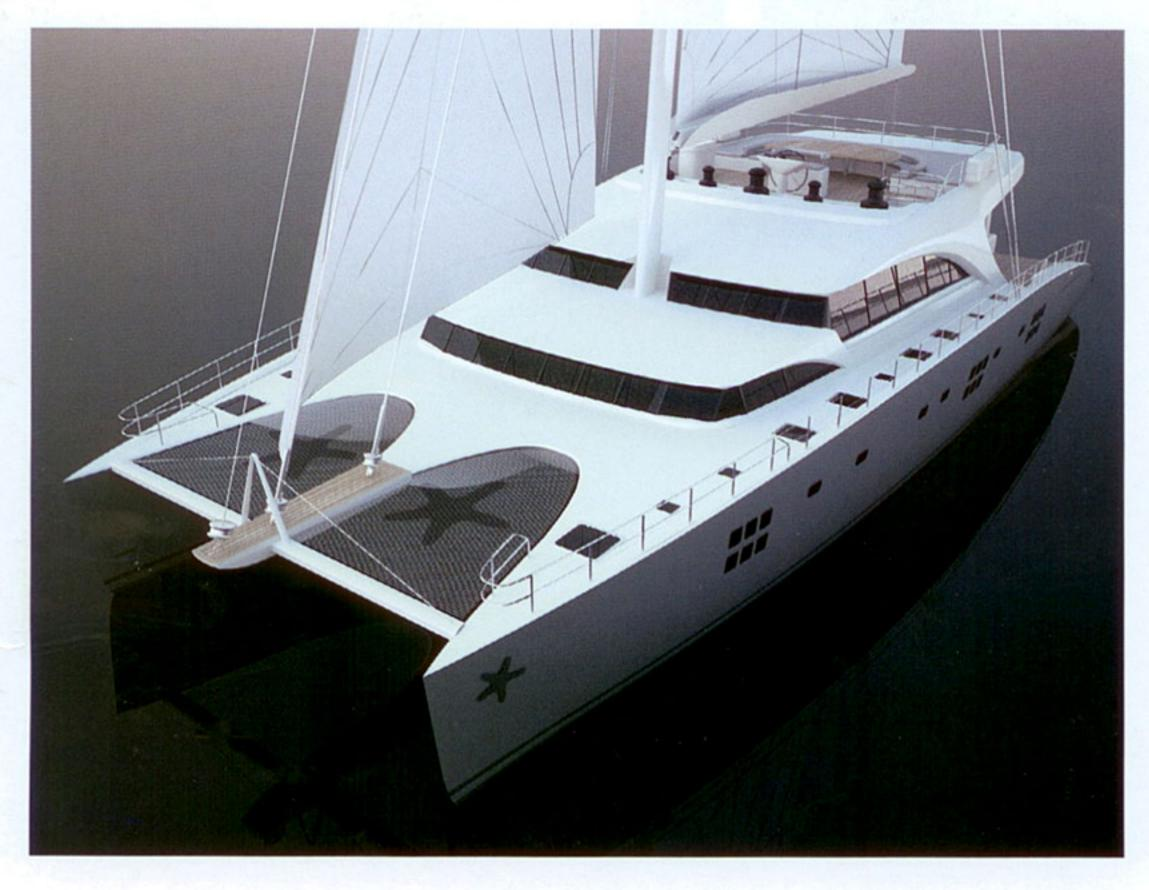
TECHNICAL DATA Length overall: 28.00 m - beam: 12.00 m - light displacement: 59,000 kilos - engines: 2x315 HP -Fuel capacity: 5,000 litres - Water capacity: 3,000 litres - Sail plan: 427 sq.m. with main and genoa, 560 sq.m. with main and gennaker - project by: Sunreef Yachts.
