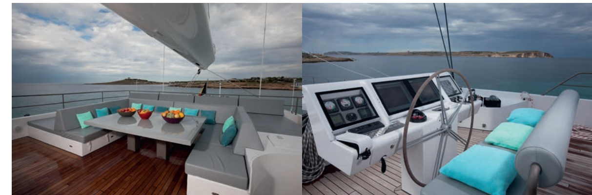
The nav station lies forward on the flybridge and affords fantastic 360 degree views. This is clearly an ideal position from which to manoeuvre the vessel and both engines, thrusters and prop pitch can be controlled from here. Che cruises easily at 12 knots on just 65 per cent engine capacity, and to conserve fuel she will make nine knots with one engine
