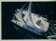
LOA 74'; LWL 68'; Beam 35'; Draft 5'8"; Displacement 78,000 lbs.; Sail area 3,17 sq. ft.; SA/D 27.8; D/L 121.4; L/BOA 2.11 Auxiliary 240-hp diesel (twin); Fuel 950 gals.; Water 316 gals.
